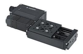
The CMLS Series Miniature Motorized Stages offer an innovative design that combines submicron precision with user-friendly operation and affordability, making them an ideal choice for programmable motion applications. These stages feature a dual-bearing design to eliminate backlash and a proprietary optical encoder, achieving nanometer-level resolution and submicron repeatability.
